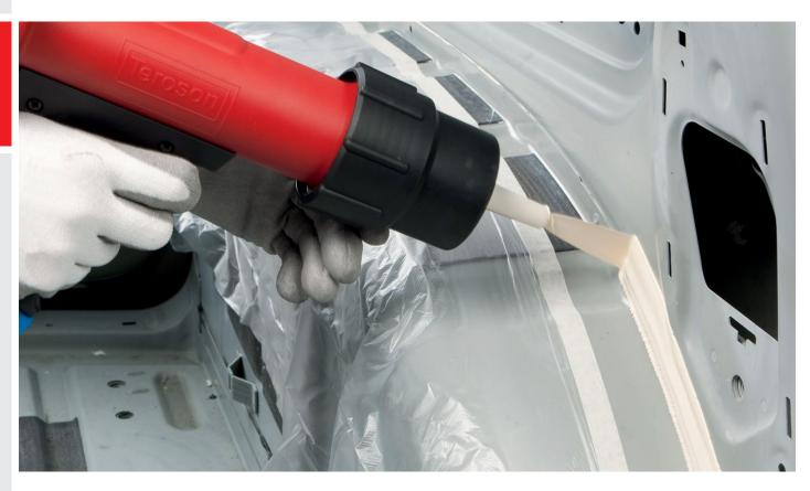
Joining methods in car bodies range from bolting, riveting, spot-welding, and clinching to bonding. Most of the joints are additionally sealed by the OEM to avoid water ingress.
