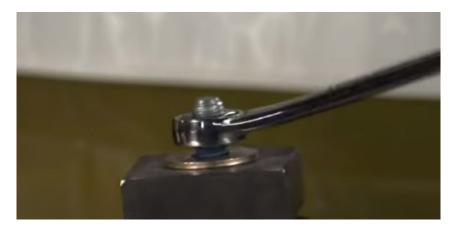
Note: As low strength & medium strength Threadlockers can be easily opened by hand tools, does not mean that they will open during vibrations. Threadlockers of any grade will never open during the vibration as the nut & bot assembly is unified addressing the root cause of gap elimination.
