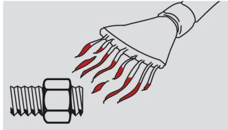
If applying heat doesn't work, switch to the chemical release method for better results. Methylene Chloride will offer optimum results.
