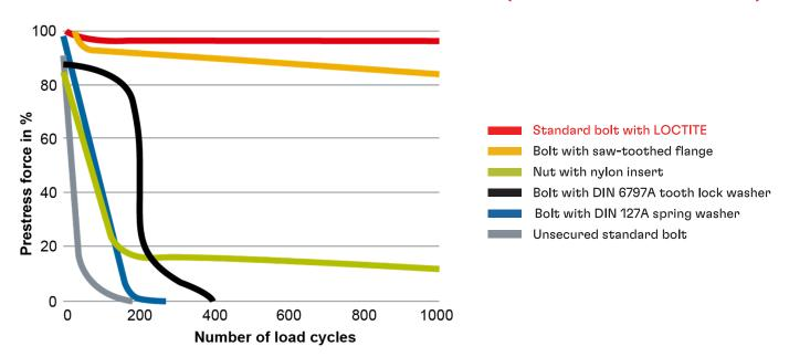
We have done Clamp Load Retention tests as shown in the above graph. Transverse shocks are given on nut & bolt assemblies to simulate the vibrational loosening. LOCTITE® Threadlocker has the best clamp load retention performance among those tested. Most traditional locking devices fail this test, resulting in loss of clamp load.
